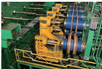
Straightening machine rollers. By updating our machinery, we have improved the dimensional and formal stability of large products
