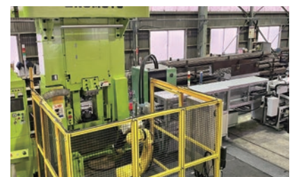
Automatic bolthead molding system
