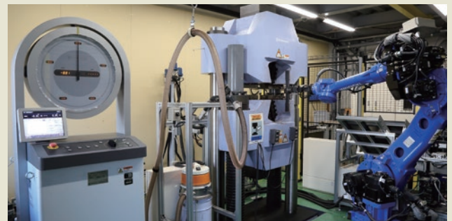
Rue tension / compression testing machine (2 MN capacity)
